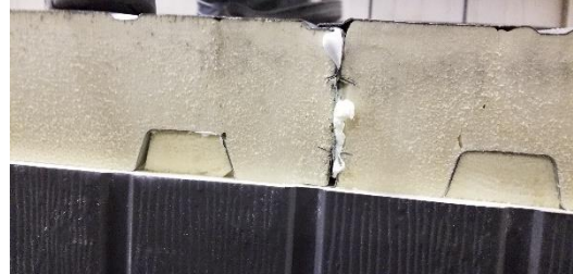
Figure 51: Acceptable Joint with proper squeeze out
