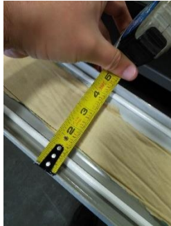
Figure 11: sealant Bead Size \frac{1}{4} "
